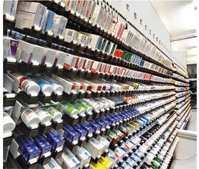
*Replenishment is logical, fast, and uncomplicated. Technicians scan the medication's bar code, enter the quantity to load, and insert medication packets. RoboPharma software guides the replenishment and tracks inventory levels.*
