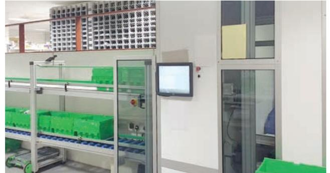
*RoboPharma's operating system steers the network of high-speed dispensing robots and integrated tote conveyors so there is no holdup or backup to each hospital ward's mini-pharmacy.*
