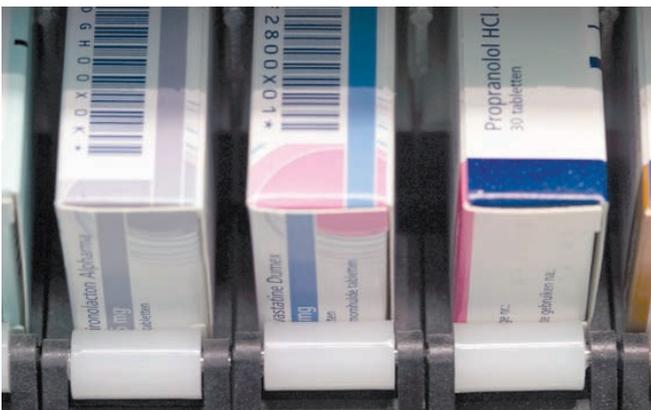
*Channel dispensing benefits include low power usage, quiet operation, and no downtime. Full access to stock is available even in a power failure or scheduled maintenance.*
